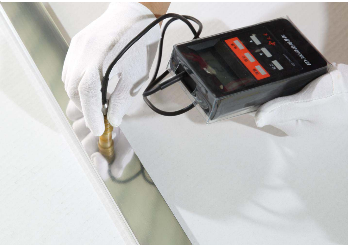
aluminium profile chrome layer thickness testing
